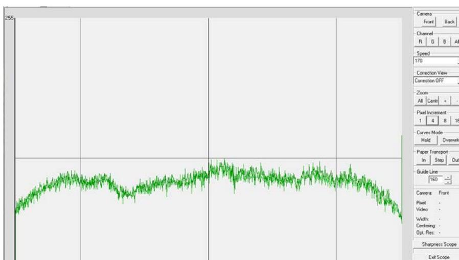
and the *Camera Scope* (figure left) is opened. The initially displayed green channel is sufficient for the adjustment, as it generates the highest values. In the menu on the right hand side **Correction OFF** must be selected as *Correction View*.
